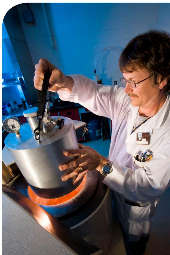
A reactor operator is analyzing a sample of air from the reactor, testing for the presence of fission gases
