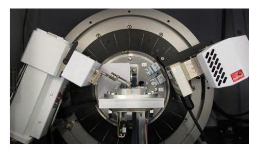
The X-ray diffraction (XRD) system is a powerful tool used to characterize crystalline materials. It permits both qualitative and quantitative analysis of minerals or other crystalline compounds present in samples.
