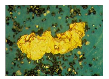
Gold prospecting by recovering, counting and examining the metallic gold grain in till samples has proven to be several magnitudes more sensitive than typical gold analysis of soils. Till samples are subject to the various gravity and magnetic processes that will extract gold grains as small as 10  $\mu$ m. Gold grains are identified using a binocular microscope.
