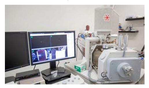
QEMSCAN® is used in mineral processing to assess the key characteristics of targeted minerals in order to design efficient recovery processes. In mineral exploration, QEMSCAN® can be used to provide quantitative modal analysis and virtual petrography on thin sections and core for target prioritization.
