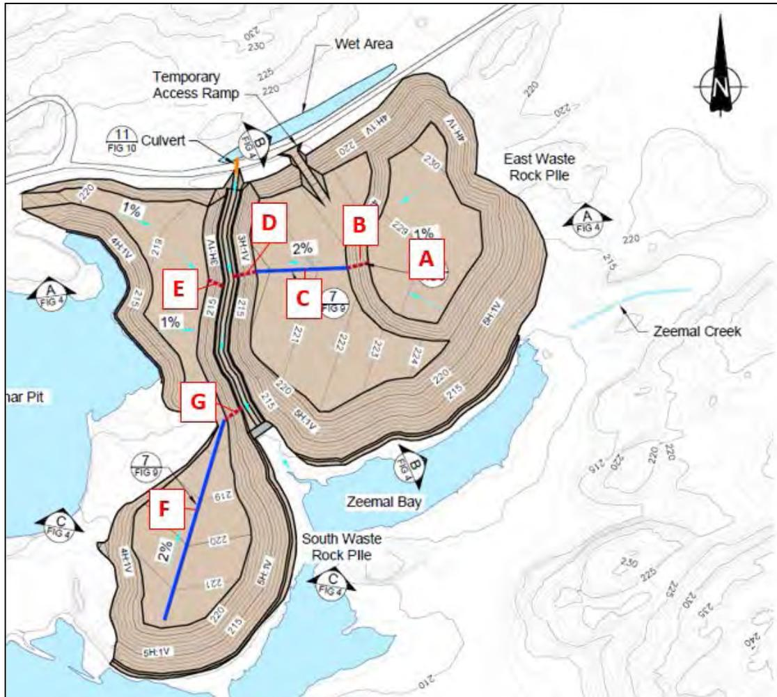
**Figure 4: Location of Waste Rock Water Conveyance Structures**
