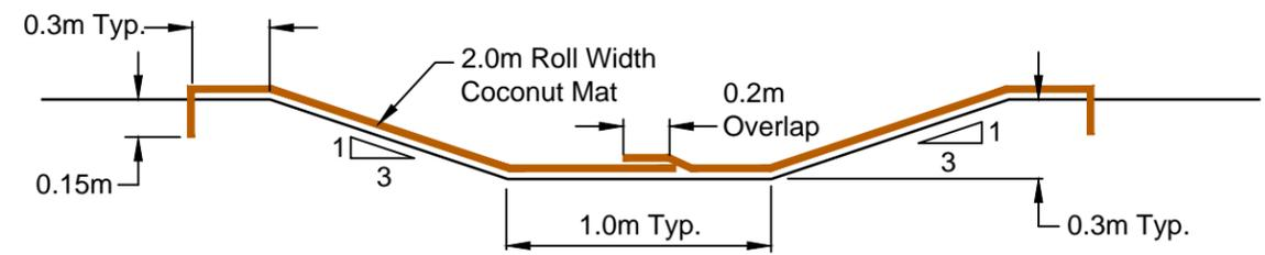
7 TYPICAL COCONUT MAT DRAINAGE CHANNEL SECTION
