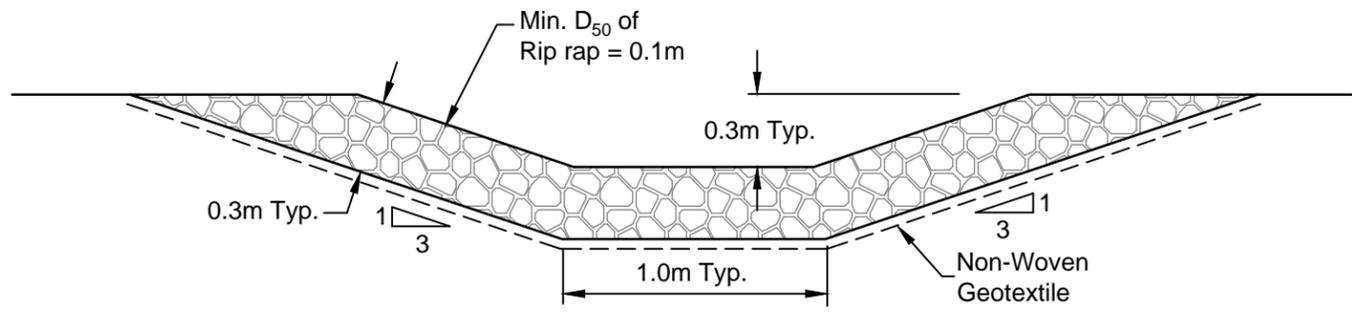
6 TYPICAL RIPRAP DRAINAGE CHANNEL SECTION
