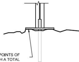
BASEPLATE TO BEAR ON 4 POINTS OF CONTACT MINIMUM WITH A TOTAL BEARING AREA OF 5200mm<sup>2</sup> (8 IN<sup>2</sup>)
