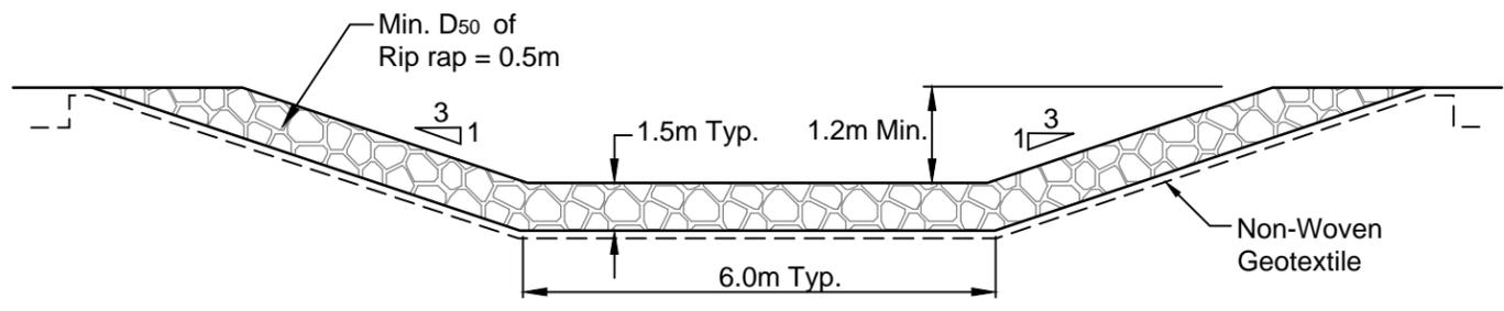
8 MAIN CHANNEL SECTION AT 13% SLOPE
