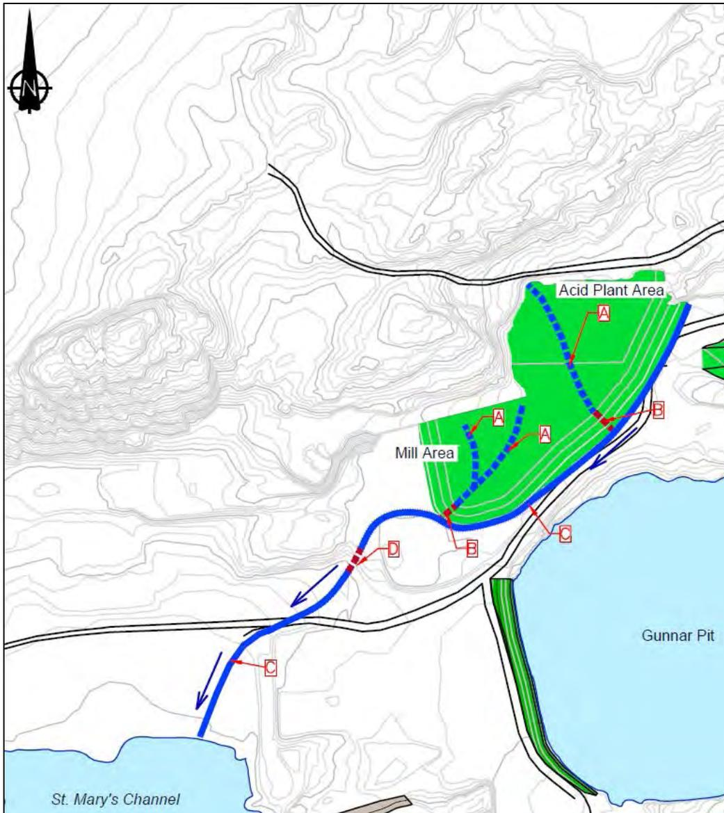
Figure 5: Location of Landfill Water Conveyance Structures
