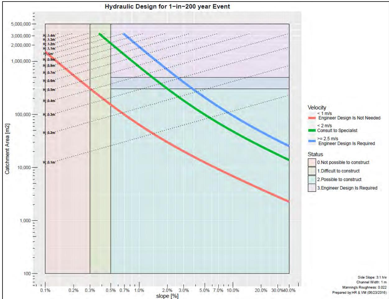
**Figure 2: Hydraulic Design Tool for Ranking Channel Features**
