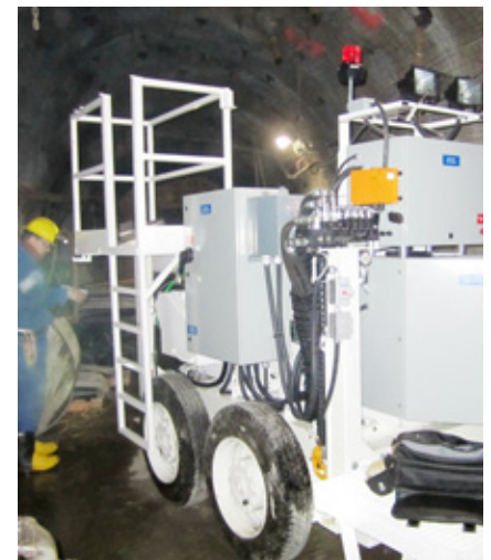
Underground Up-hole Ore Mapping System
