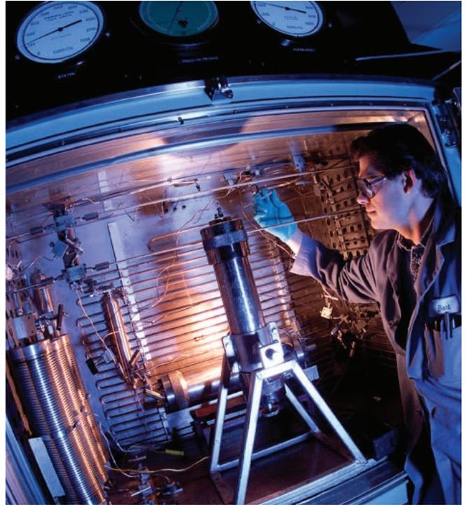
An SRC research technologist prepares the light oil coreflood apparatus for a test.
