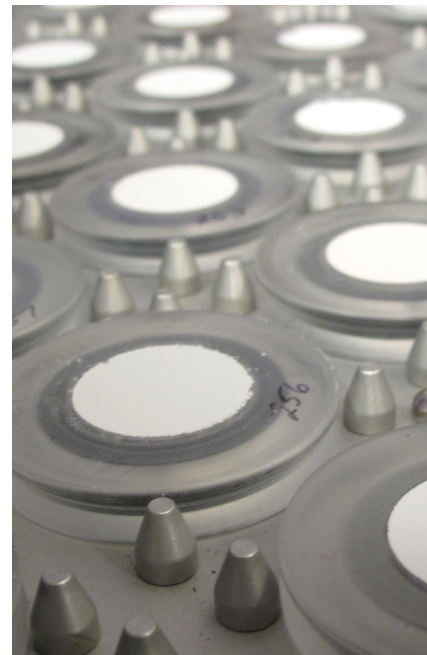
Powder samples loaded into the D4 sample magazine (max. capacity is 66 samples).
