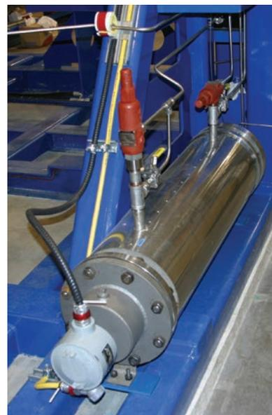
Instrumented wet test meter
