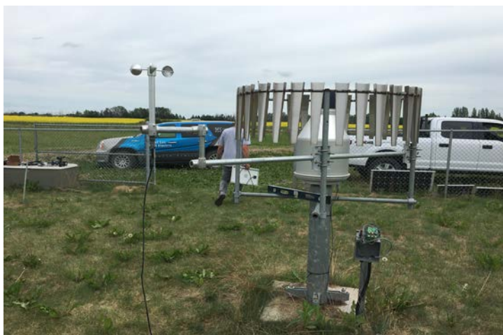
All-season precipitation weighing gauge with anemometer at 2 meter height July 2019
