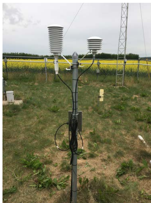
Duplicate air temperature / relative humidity sensors July 2019
