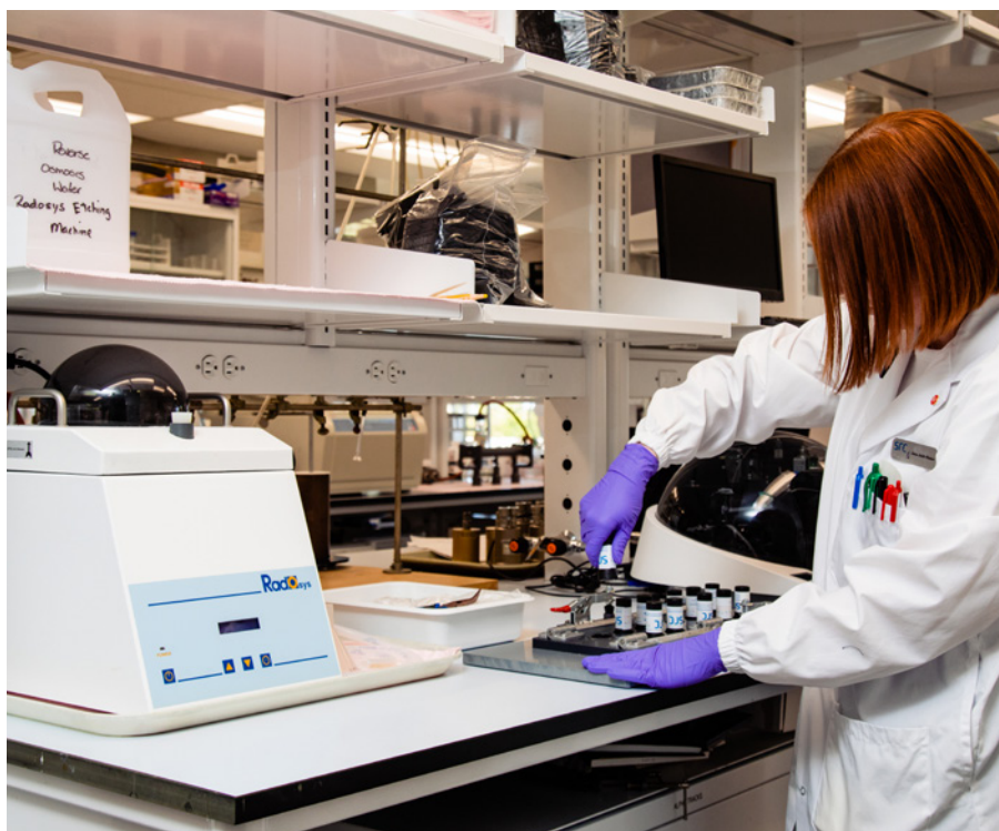
A technologist performing radon emanation rate analysis at SRC Environmental Analytical Laboratories
