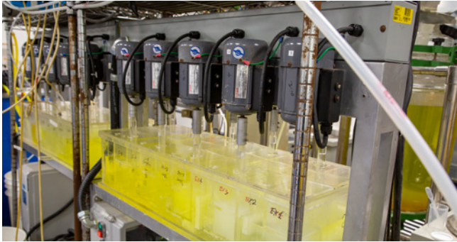
Uranium solvent extraction processing pilot equipment running a test at SRC
