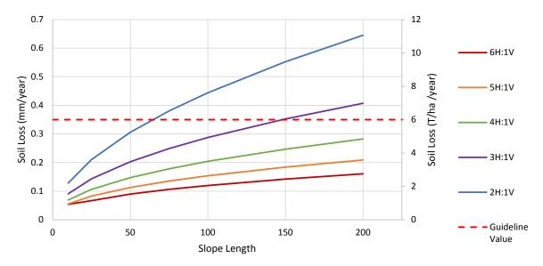
Figure 4: Straight slopes using Borrow Area 6W Material with 40% small, short-rooted plant coverage and no vegetative canopy
