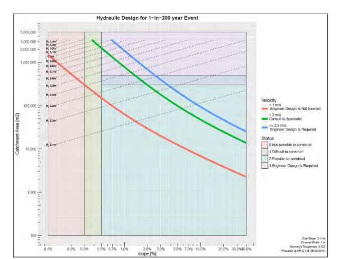
Figure 2: Hydraulic Design Tool for Ranking Channel Features
