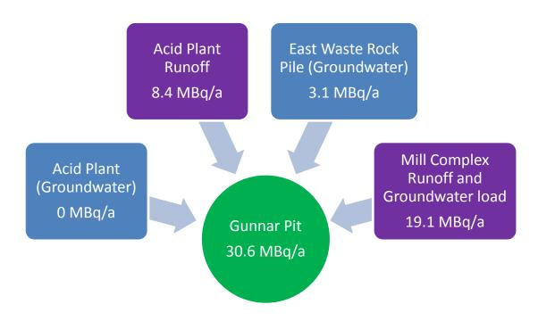
Figure 30: Schematic of Radium-226 Loads to Open Pit Associated with Remedial Actions
