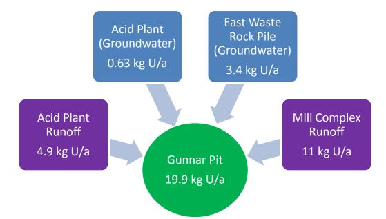
Figure 6: Schematic of Current Uranium Loads to Gunnar Pit
