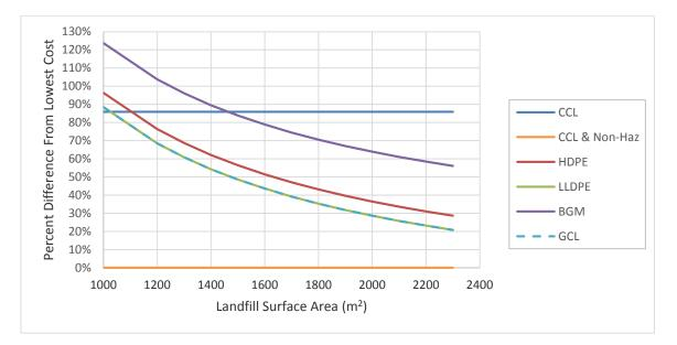
Figure 1: Comparative Cover Cost versus landfill surface area.
