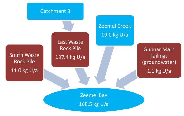
Figure 8: Schematic of Current Uranium Loads to Zeemel Bay
