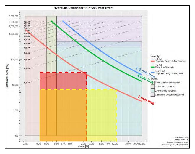
Figure 3: Example Use of the Hydraulic Design Tool
