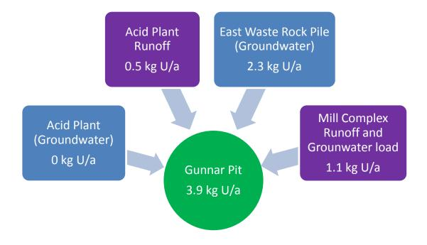
Figure 29: Schematic of Uranium Loads to Open Pit Associated with Remedial Actions
