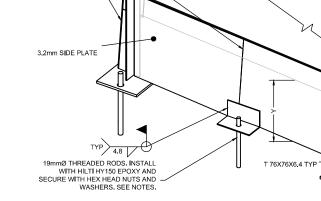
NOTE: SIDE CLIPS REQUIRED IF Y>380mm OR X >1.4m
