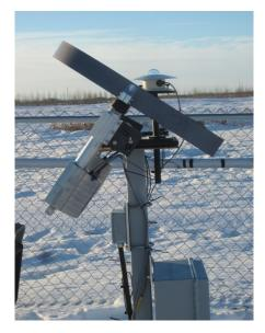
Automated shade ring for diffuse pyranometer 17 Jan 2014 photo credit: DE&M, SRC
