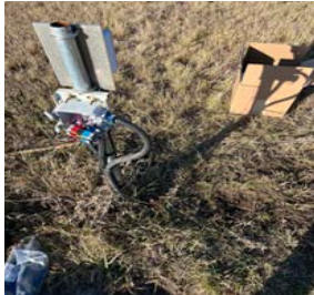
Replacement of 20cm soil moisture sensor Oct 2024 Photo: K. Babich
