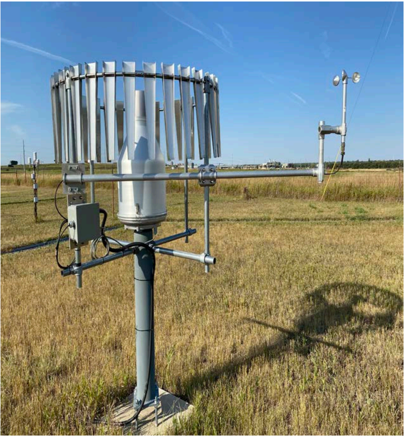
All-Season Precipitation Weighing Gauge with 2 meter anemometer 27 August 2024 Photo: V. Wittrock
