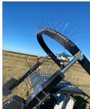
Auto-movement Ring to shade Diffuse Pyranometer 08 October 2024 Photo: V. Wittrock
