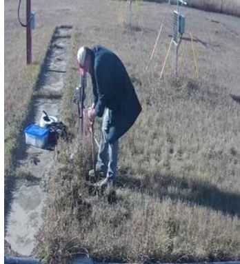
Replacement of 20cm soil moisture sensor Oct 2024 Photo: V. Wittrock
