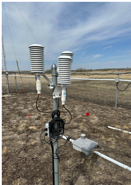
Air temperature / relative humidity sensors Apr 2024 Photo: R. Jansen
