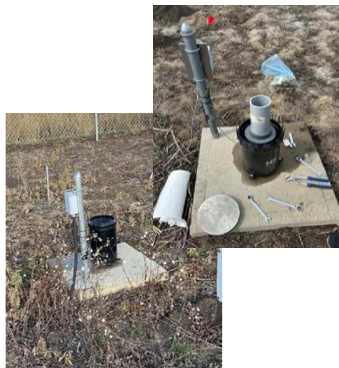
Tipping Bucket liquid precipitation gauge (Spring and fall maintenance) April 30 2024 and October 31 2024 Photo: R. Jansen and K. Babich
