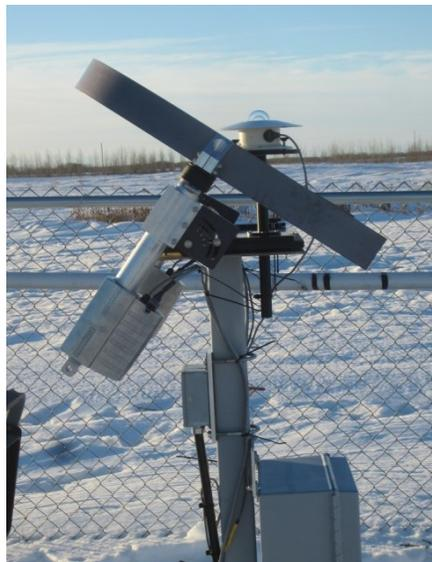
Automated shade ring for diffuse pyranometer
