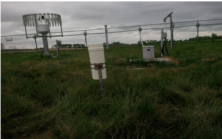
Weighing Gauge, AES Standard Manual Gauge,
