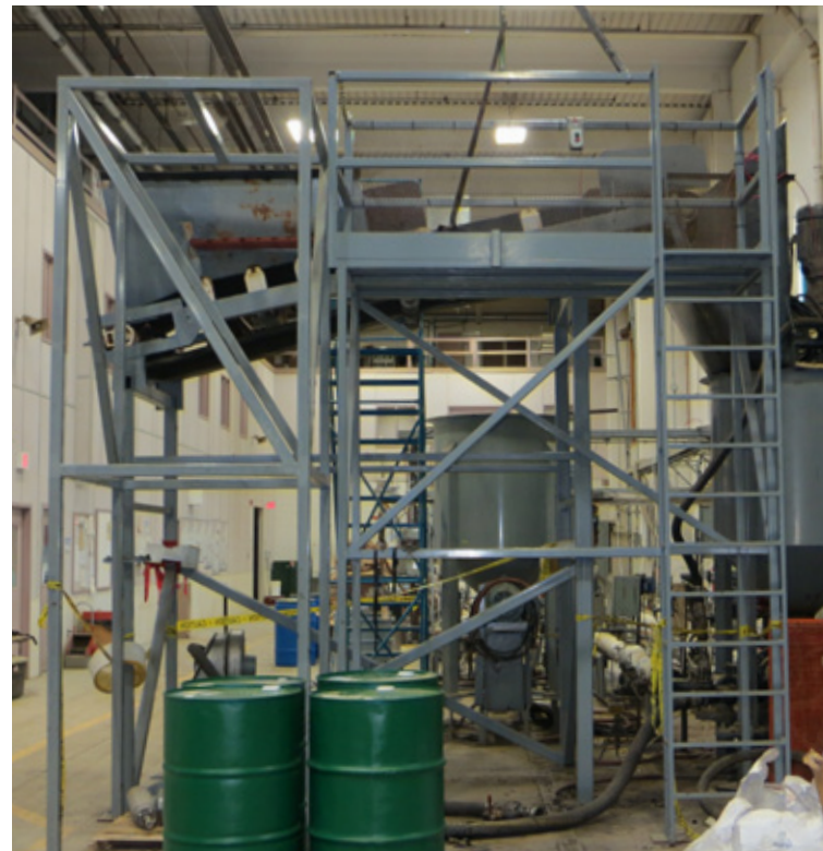
Experimental Work Platform for Conveyor Operation – Designed and Built In-house
