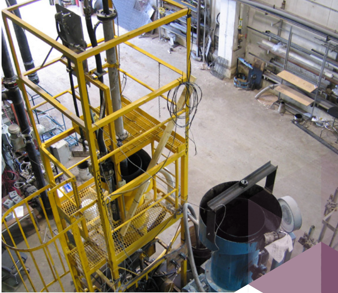
Pilot-Scale Hydrocyclone and Thickener Equipment Pilot
