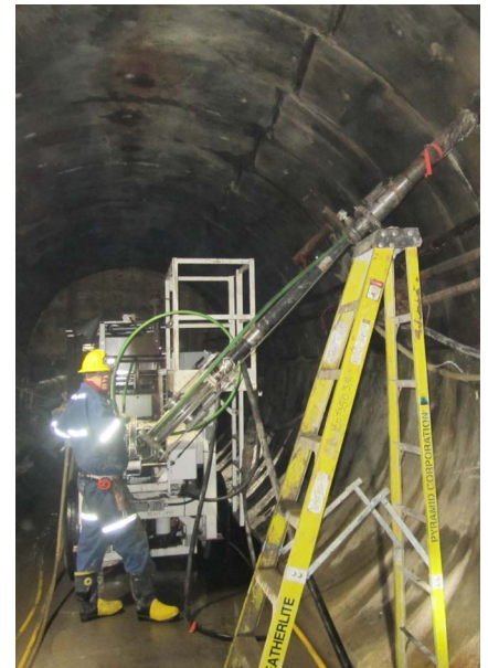
BHASS during surveying. Gamma probe and inertial probe were used to map this borehole. Probes were loaded into a borehole from an elevated platform located on the BHASS.
