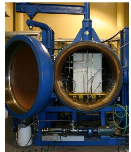
3-D physical model in pressure vessel. SRC's sealed, explosion-proof SVX laboratory is certified as Class 1, Zone 2 by the Canadian Standards Association.
