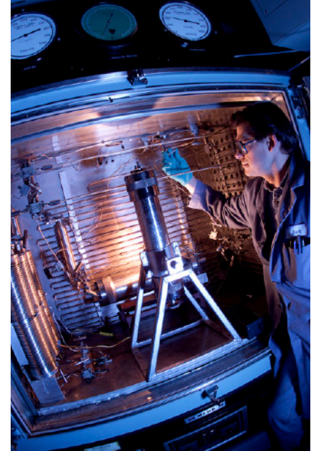
An SRC research technologist prepares the light oil coreflood apparatus for a test.
