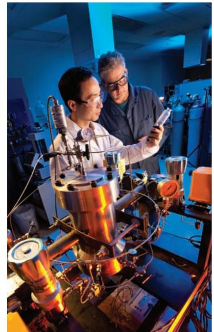
Examining samples from a radial coreflood apparatus.
