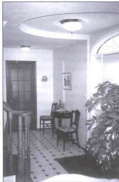
The ceiling light fixtures use compact fluorescent lamps. Ceramic tile flooring avoids offgassing from vinyl floors.
