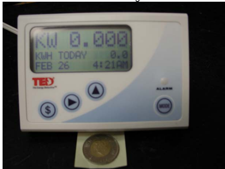
Figure 3. The Energy Detective Readout Device (A 2 dollar coin is shown below the unit for scale.)
